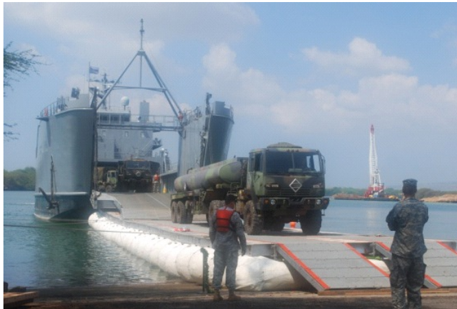
FIG. 1. Prototype for rapidly deployable causeway system. Image courtesy of US Army ERDC.
