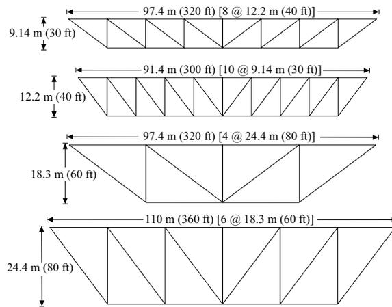
**FIG. 5. Elevation views of the four combinations of Pratt trusses evaluated.**
