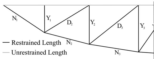
**FIG. 7. Partial elevation view of bowstring truss form.**
