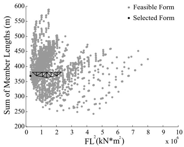
**FIG. 8. Selection of bowstring truss form: Comparison of total length of panels to structural performance metric ( $FL^2$ ). The selected form is sketched.**
