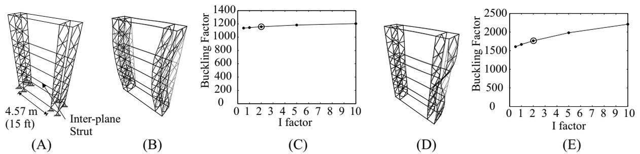
**FIG. 13. Parametric study of inter-plane bracing in a column-like configuration, including (A) isometric view indicating boundary conditions, (B) buckled shape under vertical load (for selected option), (C) buckling factor under vertical load as a function of I factor (selected option is highlighted) (D) buckled shape under horizontal load (for selected option), and (E) buckling factor under horizontal load as a function of I factor (selected option is highlighted).**
