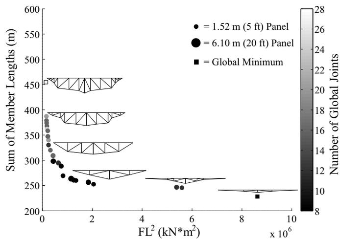
**FIG. 16. Results of multi-objective optimization procedure for the bowstring truss form. Marker size indicates the number of panels and grayscale coloring indicates the number of global nodes. Global minima included for reference.**
