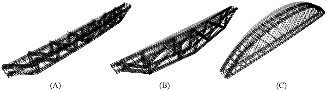
**FIG. 15. Buckled shapes of the new bridge forms: (A) Pratt truss, (B) bowstring truss, and (C) network tied arch.**
