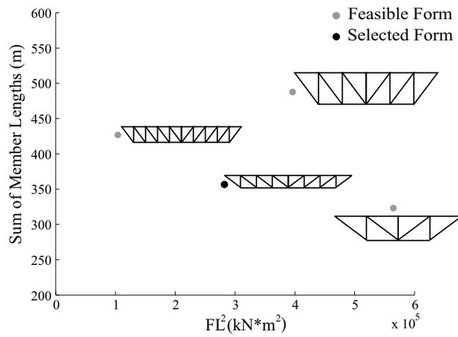
**FIG. 6. Selection of Pratt truss form: Comparison of total length of panels to structural performance metric ( $FL^2$ ). All feasible forms are sketched.**
