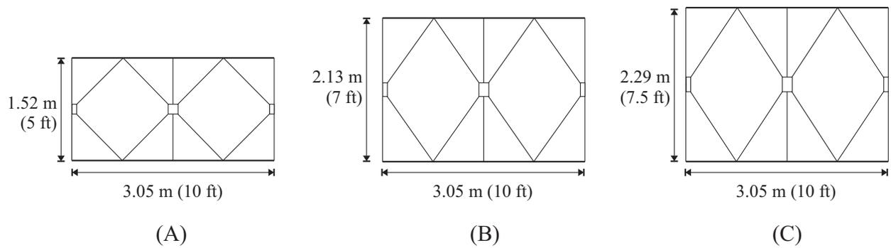
**FIG. 1. Elevation views of (A) Bailey [Standard US Army M2 (Pioneer Bridges, a Division of Bailey Bridges, Inc., 2015)], (B) Mabey Johnson [Compact 200 (Mabey, 2015)], and (C) Acrow [700XS, (Acrow Corporation of America, 2009)] panels.**
