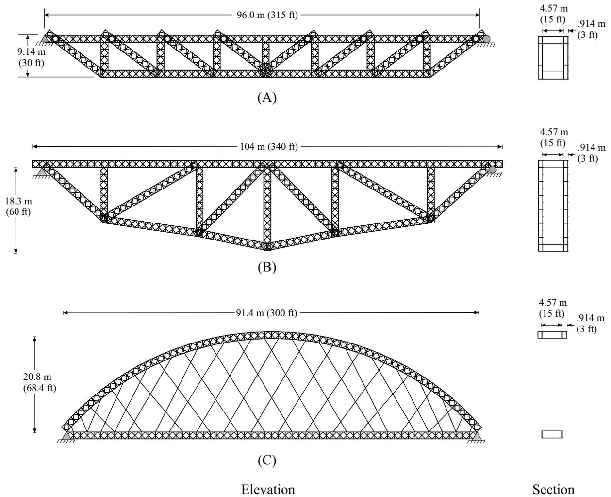
**FIG. 14. New bridge forms in elevation view (left) and section view (right): (A) Pratt truss, (B) bowstring truss, and (C) network tied arch.**
