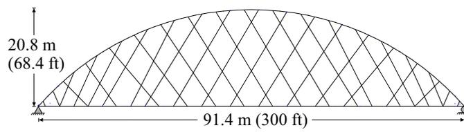
**FIG. 9. Elevation of network tied arch form.**
