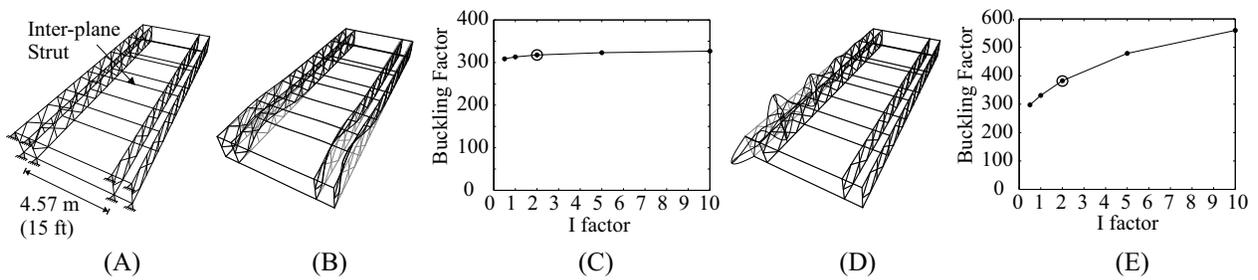
**FIG. 12. Parametric study of inter-plane bracing in a girder-like configuration, including (A) isometric view indicating boundary conditions, (B) buckled shape under vertical load (for selected option), (C) buckling factor under vertical load as a function of I factor (selected option is highlighted) (D) buckled shape under horizontal load (for selected option), and (E) buckling factor under horizontal load as a function of I factor (selected option is highlighted).**
