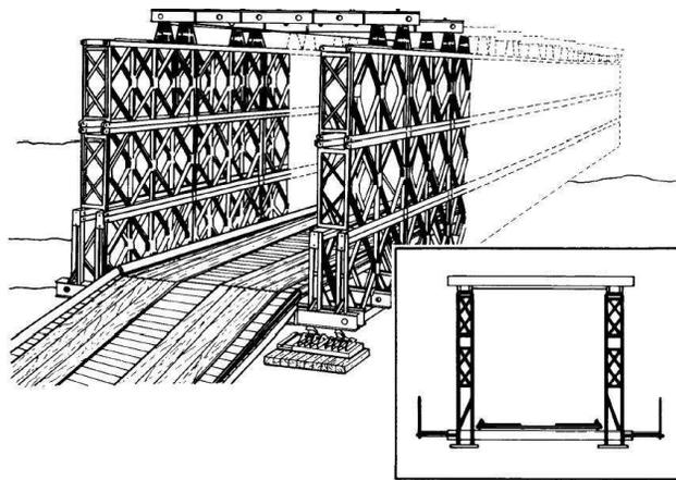
**FIG. 2. Double-triple configuration of Bailey Bridge panels, including isometric and section views. Images courtesy of US Army (Department of the Army, 1986).**
