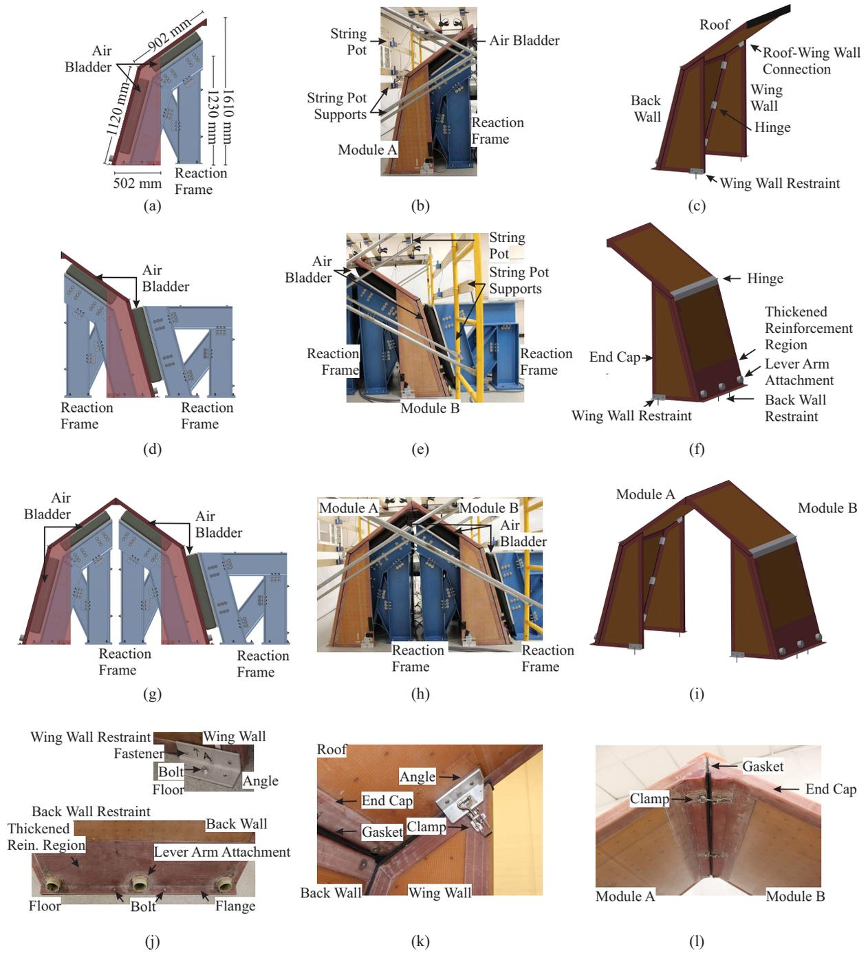
FIG. 4: Module A test: (a) elevation view, (b) photograph, and (c) isometric view; Module B test: (d) elevation view, (e) photograph, and (f) isometric view; Two Module test: (g) elevation view, (h) photograph, and (i) isometric view; Photographs of connection details: (j) ground restraints for wing walls and back walls, (k) connection between wing wall and roof, and (l) roof connection between modules.
