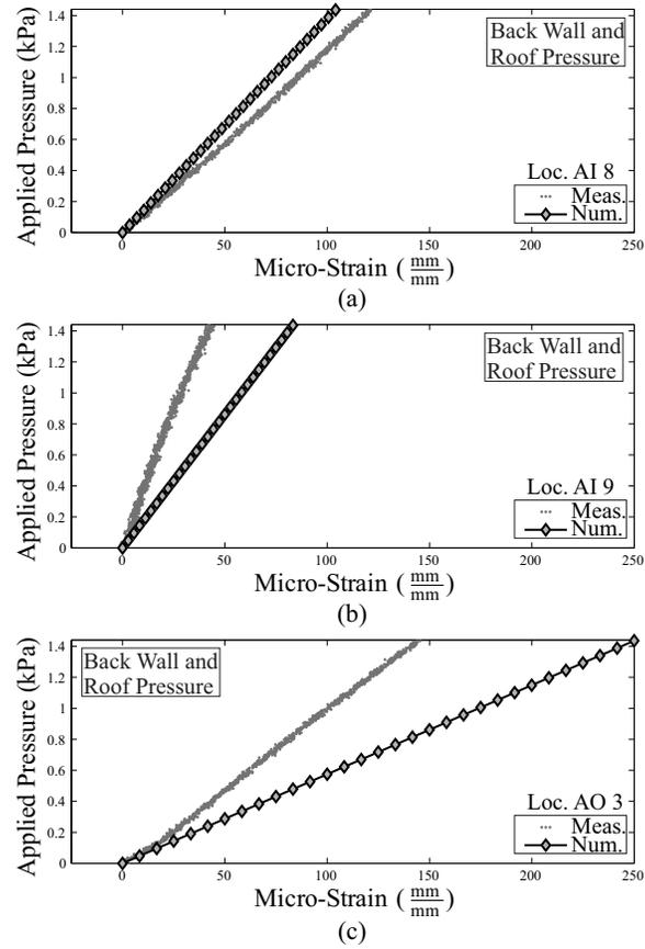
FIG. 10: Module A test: measured and numerical surface strains at (a) roof near roof-wing wall connection, (b) at wing wall near roof-wing wall connection, and (c) and at wing wall near ground restraint when pressure applied to back wall and roof simultaneously.
