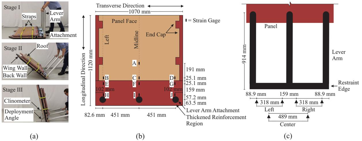
FIG. 3: Deployment test: (a) photograph, (b) plan view of measurement system on back wall, and (c) plan view of varying hand positions on lever arm.
