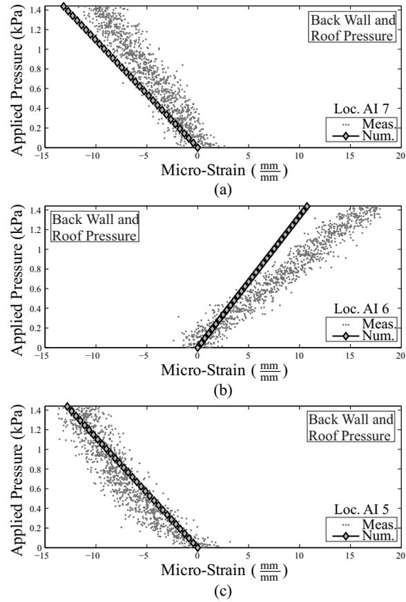
FIG. 11: Module A test: measured and numerical surface strains at back wall for pressure applied to the back wall and roof at (a) top hinge, (b) middle hinge, and (c) bottom hinge.
