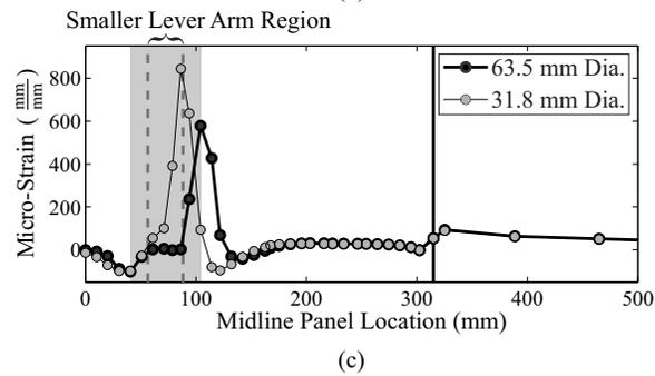
FIG. 7: Impact of (a) length of reinforcement region, (b) number of lever arm attachments, and (c) diameter of lever arm on behavior during deployment: Numerical longitudinal surface strains at deployment angle  $\theta = 5^\circ$  along longitudinal length of panel.
