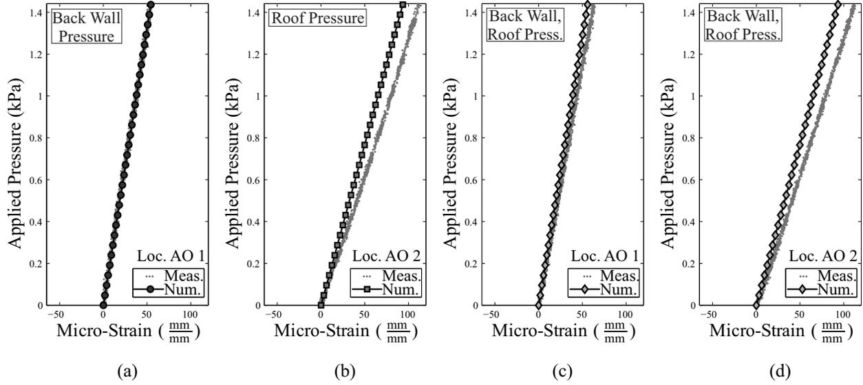
FIG. 9: Module A test: measured and numerical surface strains for pressures applied to (a) back wall (strain at center of back wall), (b) roof (strain at center of roof), (c) back wall and roof (strain at center of back wall), and (d) back wall and roof (strain at center of roof).
