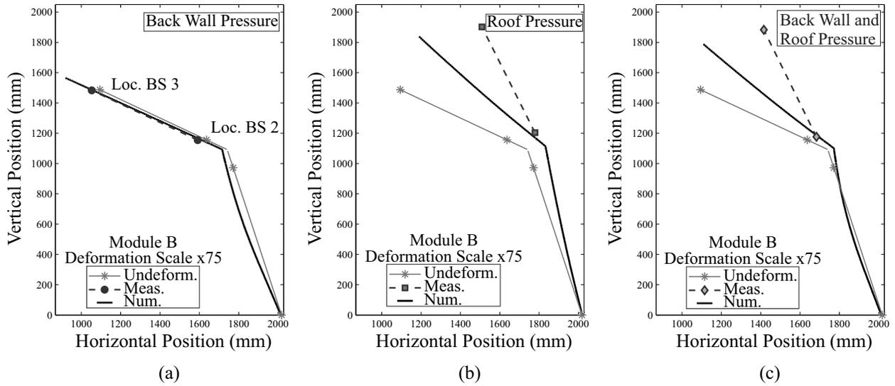
FIG. 12: Module B test: measured and numerical deformed profiles for pressures applied to (a) back wall, (b) roof, and (c) back wall and roof, compared against the undeformed (undeform.) shape. Measured data is connected by dashed, straight lines for reference and deformations are multiplied by scale factor of 75 for clarity.
