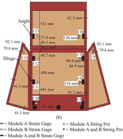
FIG. 5: Module tests: plan view of measurement system shown in a flat (i.e., undeployed) configuration on the (a) outside, and (b) inside surfaces.
