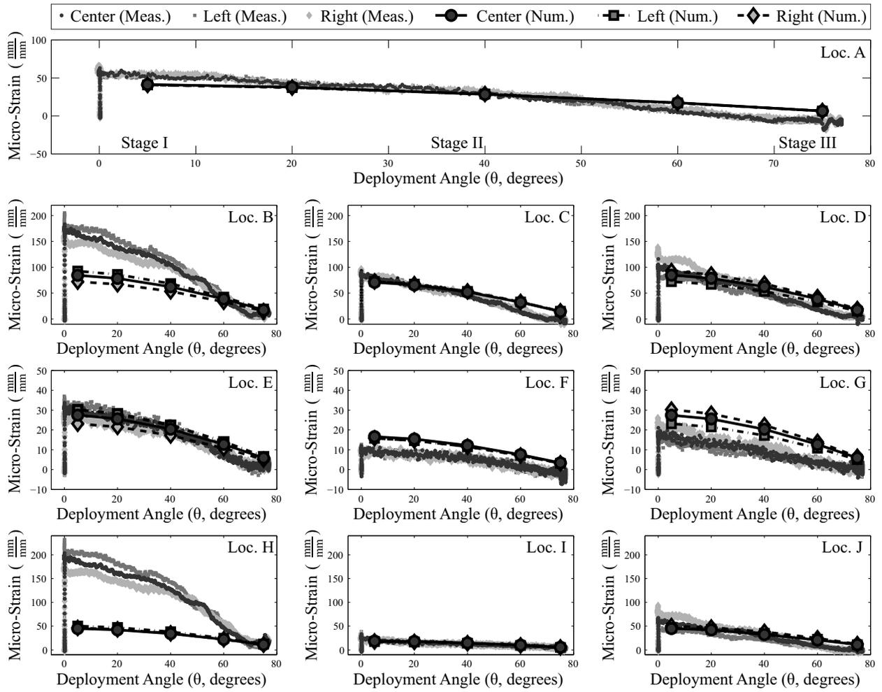
FIG. 6: Measured and numerical longitudinal surface strains during deployment for hand positions at center, left, and right on lever arm.
