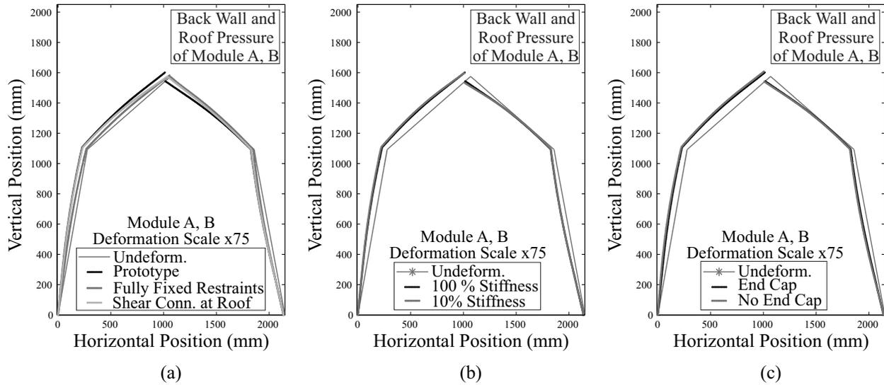
FIG. 16: Impact of (a) restraints and the connection between modules, (b) stiffness of gasketing, and (c) end cap reinforcement on deformed shape for pressures applied to back wall and roof of both Modules A and B. Deformations are multiplied by scale factor of 75 for clarity.
