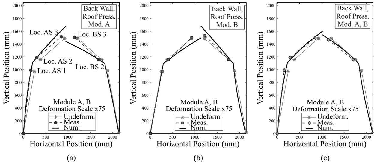
FIG. 14: Two Module test: measured and numerical deformed profiles for pressures applied to (a) back wall and roof of Module A, (b) back wall and roof of Module B, and (c) back wall and roof of both Modules A and B, compared against the undeformed (undeform.) shape. Measured data is connected by dashed, straight lines for reference and deformations are multiplied by scale factor of 75 for clarity.
