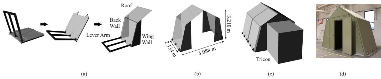
FIG. 1: Origami-inspired deployable shelter developed by Quaglia et al. (2014a): (a) deployment, (b) two modules with dimensions, (c) complexed, enclosed modules with a Tricon container, and (d) full-scale deployed prototype. Images (a)-(c) reprinted from Ballard et al. (2016).
