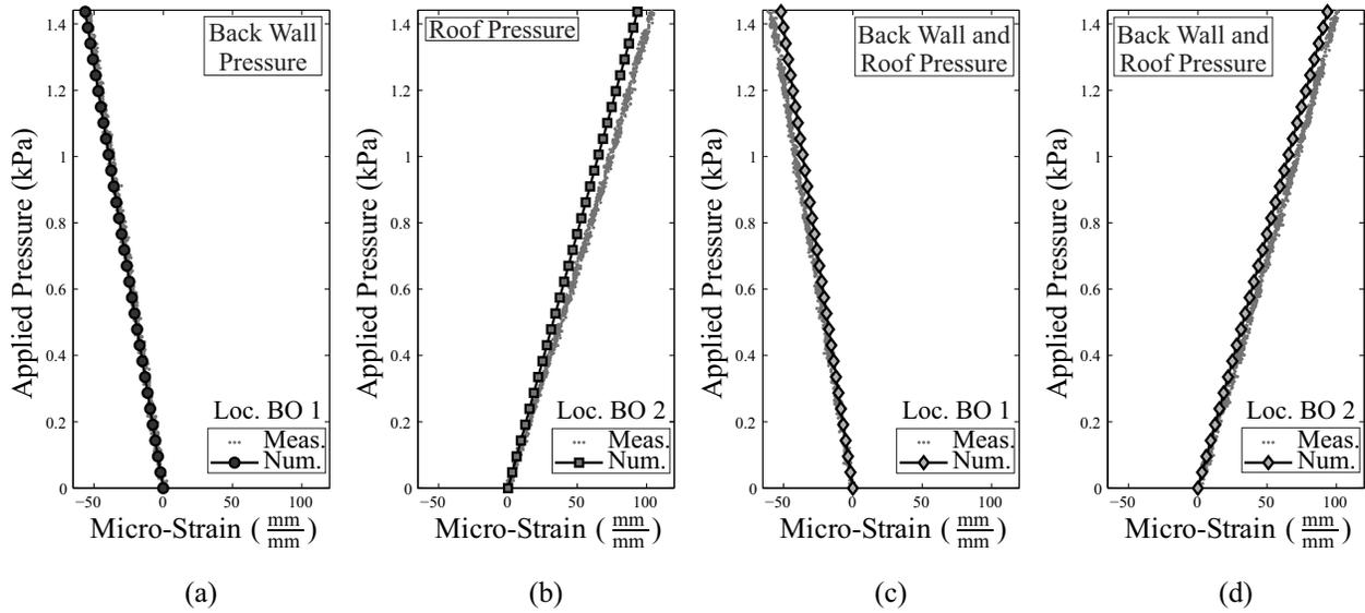
FIG. 13: Module B test: measured and numerical surface strains for pressures applied to (a) back wall (strain at center of back wall), (b) roof (strain at center of roof), (c) back wall and roof (strain at center of back wall), and (d) back wall and roof (strain at center of roof).
