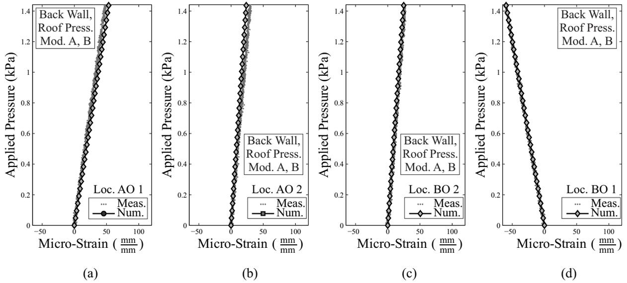
FIG. 15: Two Module test: measured and numerical surface strains for pressures applied to back wall and roof of both Modules A and B at (a) center of back wall of Module A, (b) center of roof of Module A, (c) center of roof of Module B, and (d) center of back wall of Module B.
