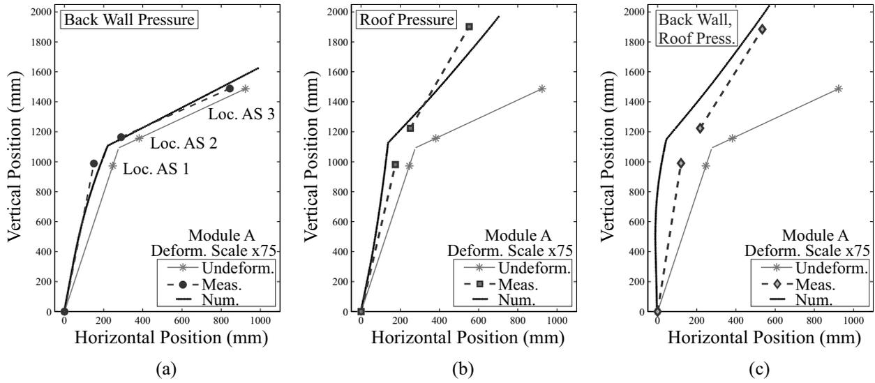
FIG. 8: Module A test: measured and numerical deformed profiles for pressures applied to (a) back wall, (b) roof, and (c) back wall and roof, compared against the undeformed (undeform.) shape. Measured data is connected by dashed, straight lines for reference and deformations are multiplied by scale factor of 75 for clarity.
