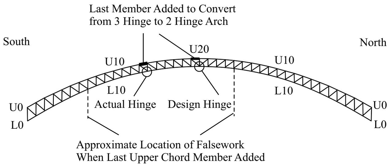
Figure 7: Joint Labeling Scheme. *This figure shows Ammann's labeling system for the joints of chords. U refers to the upper chord and L refers to the lower chord. Joint 20 is at the crown and Joints 0 are at the hinges. The joints have been individually labeled at intervals of 10. Key members and the location of the design and actual hinges have been highlighted [Troelsch 1931].*
