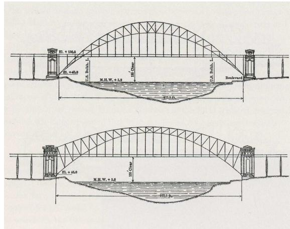
Figure 3: Lindenthal's Arch Designs. *These images are Lindenthal's sketches for the crescent form (top) and the spandrel form (bottom) (courtesy of the ASCE, Source: "The Hell Gate Arch Bridge and Approaches of the New York Connecting Railroad Over the East River in New York City," [Ammann 1918a]).*
