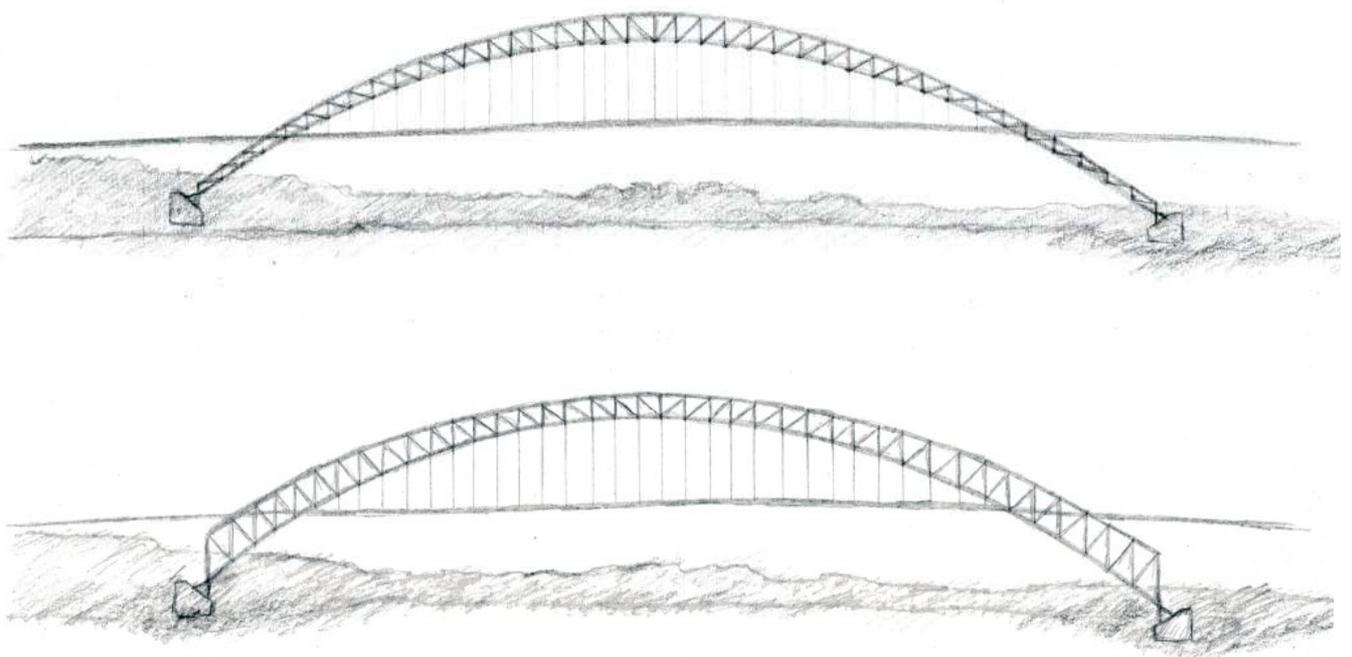
Figure 4: Sketch of Bayonne as a Crescent Form. *The top sketch is of the Bayonne Bridge as designed by Ammann. The bottom sketch is our sketch of the Bayonne Bridge if designed as a crescent arch (Source: sketches by Marilyn Parkinson Thrall and Ashley Thrall).*
