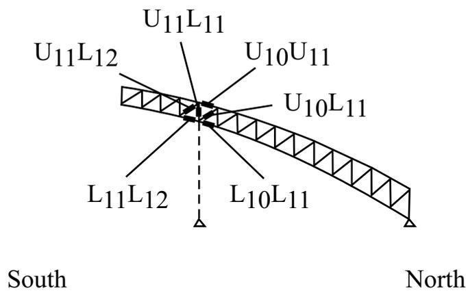
Figure 8: Construction Sketch. *This sketch represents a phase of the construction where the falsework is the column (marked by dashed lines) which is connected at Joint  $L_{11}$ . The members for which original calculations were available are labeled [Ammann 1930c].*
